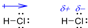
Figure 8. A Cross-base Arrow or Delta Plus/Minus Symbols Represent Bond Polarity in Hydrogen Chloride.
