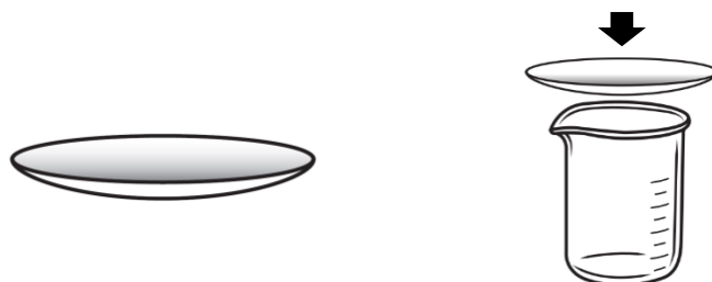
Figure 9. Watch Glass and Placement on Beaker.
