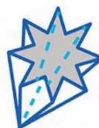
Figure 7. Open fluted (or fan-folded) filter paper
