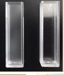
Insert the cuvette containing the blank in the cuvette chamber: place it flush to the right side, frosted side of cuvette facing you so the clear sides are aligned with the direction of the light beam.
