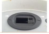
Press to zero out the instrument.
