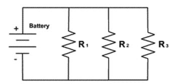
a) Calculate the equivalent resistant of the parallel circuit.
