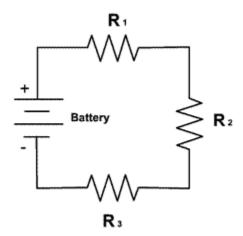
a) Calculate the equivalent resistant of the series circuit.
