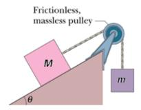
Your final equation should be:  $\underline{a=(mg-Mgsin\theta)/(m+M)}$ . You are going to use this equation to calculate the dynamical acceleration in the lab.
